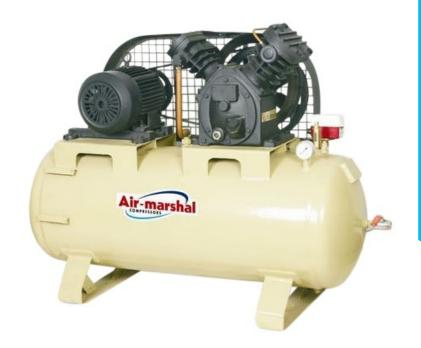
The Air-marshal two stage compressor consists of two or more cylinders. The atmospheric air enters into the LP cylinder through an inlet filter & valve which passes to the HP cylinder through the inter-cooler for a final pressure.
